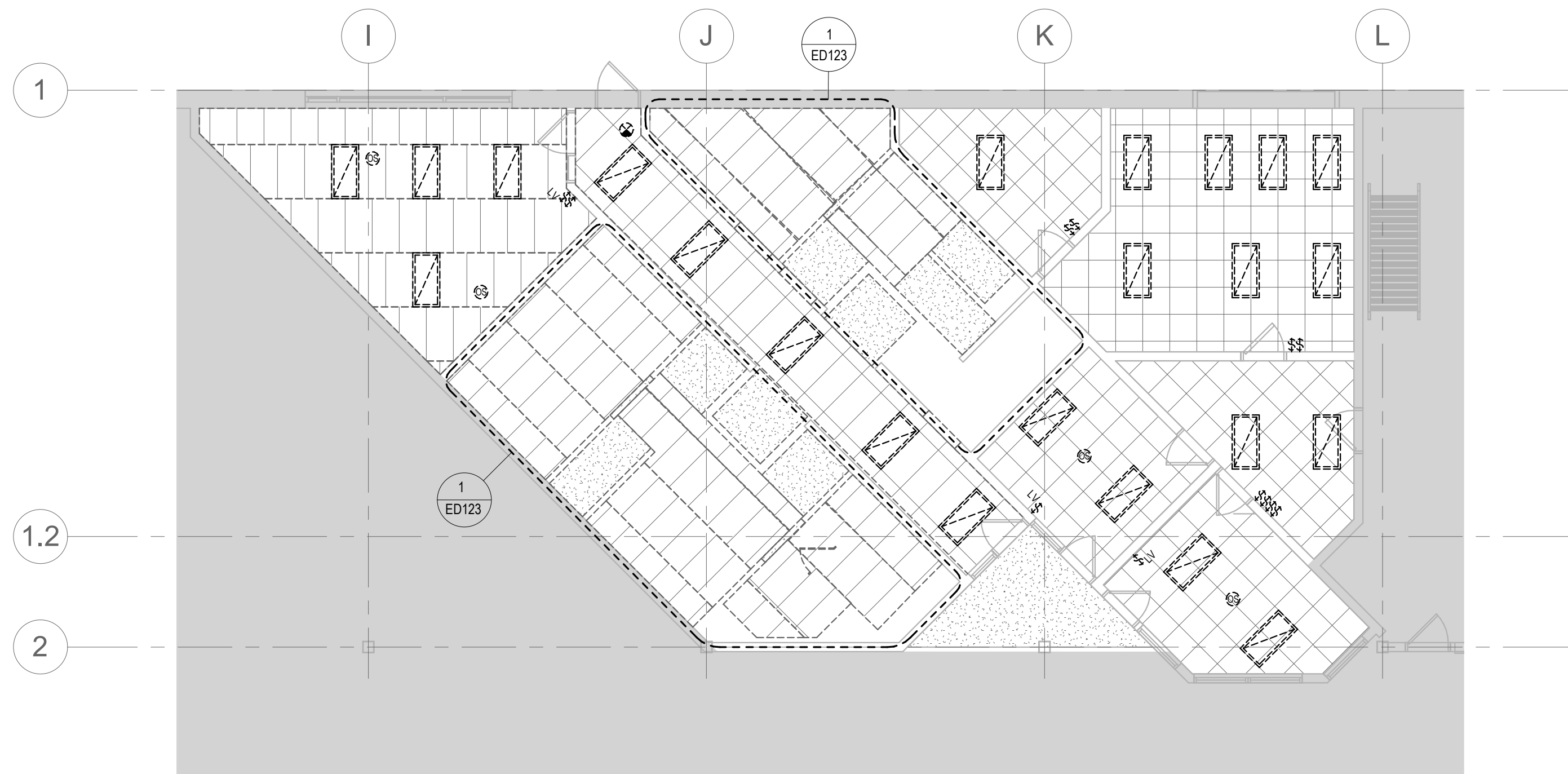
1 LEVEL 1 MECHANICS AREA LIGHTING DEMOLITION PLAN 1/8" = 1'-0"
