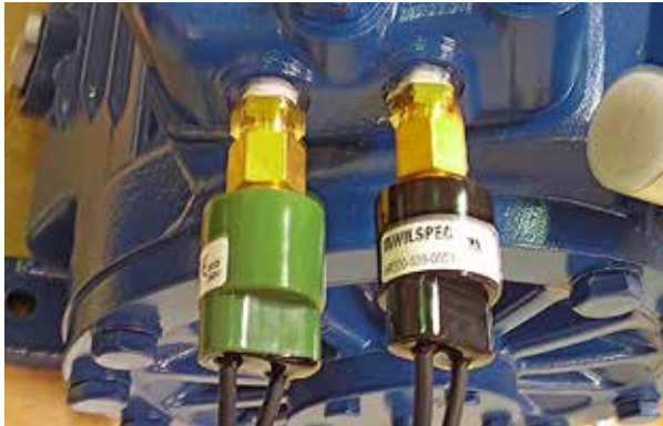
Pressure switch screw adapter installed on compressor
