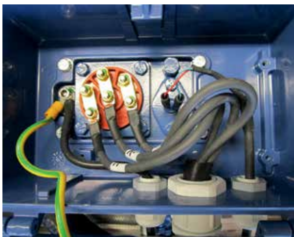
Example of a delta circuit
