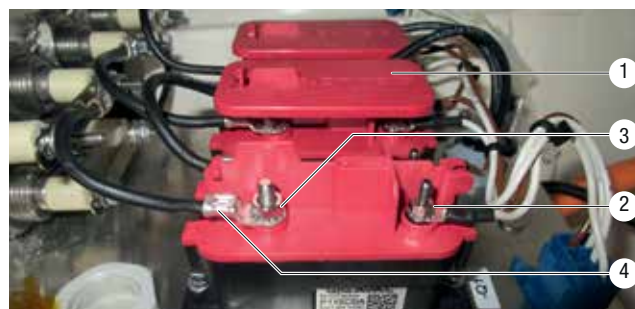
Removal of the Gigavac switching devices
