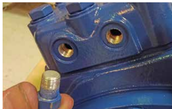
Removing sealing plugs
