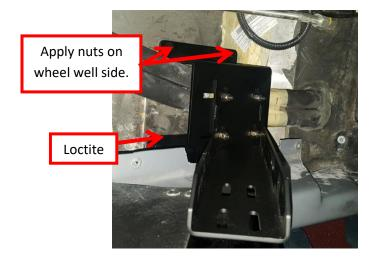
15. Check the alignment of the holes in the bus wall and the hinge mount assembly to ensure they line up. Adjust the hinge mount assembly as needed.
