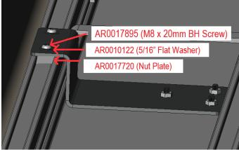
20. Locate (1) AR0017717 (Welded Pole Mounting Plate), (1) AR0017715 (Pole Mounting Plate Upper Sub-Assembly), (3) AR0010122 (5/16" Flat Washer), and (3) AR0010003 (5/16-18 Lock Nuts) and fasten together as shown. Next Slide it on top of the doors hinge post. **Tighten to a final torque of 11 ft-lbs.**
