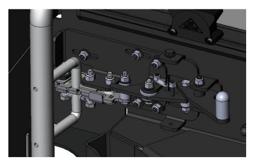
29. Mark the 4 holes on the stanchion base plate and the stanchion can be removed.
