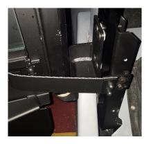
42. Locate AR0014276 (Hinge Mount Cover) and (3) 0000422F (Torx Pan Head Screws). Fasten the hinge mount cover to the hinge mount weldment as shown using the above hardware.
