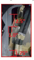
10. Behind the driver seat, drill out the upper left and middle rivet for the mounting bracket. Mark the rivet head with a center punch and drill a 1/8" Pilot Hole. Enlarge the pilot hole with a #F drill bit (0.2570") and then tap the hole with a 5/16-18 tap. Only the top rivet needs to be tapped. The middle rivet needs to be removed so the bracket sits flat over the fender wall.
