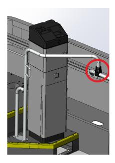
32. Use (4) AR0010117 ( $\frac{1}{4}$ "-20 Hex Bolts), (8) AR0007440 ( $\frac{1}{4}$ " Flat Washers), and (4) AR0004824 ( $\frac{1}{4}$ -20 Lock Nuts) to secure the stanchion to the farebox pedestal. **Tighten to a final torque of 7 ft-lbs.**
