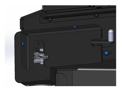
40. Locate AR0011243 (Tether Retainer) and AR0014279 (Tether Adjuster). Position the adjuster on the backside of the strap and the Retainer on the front. Use (2) AR0012529 (¼-20 x 1" FH Screws), (2) AR0007440 (1/4" Flat Washers), and (2) AR0004824 (¼-20 Lock Nuts) to fasten the 3 pieces together. Place AR0011048 (1/4" Dome Cap) over the nut. **Tighten to a final torque of 7 ft-lbs.**
