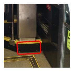
27. Locate AR0023776 (Stanchion Weldment) and AR0011994 (Handrail Clamp). Position the stanchion 1/2" from the driver pedestal as shown below and use the handrail clamp to attach the stanchion to the front handrail.
