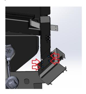
25. Locate AR0014565 (Hinge Closeout), (4) AR0014566 (¼"-20 x 1.25" BH Screws), (4) AR0007440 (¼" Flat Washers), and (4) AR0007439 (1/4"-20 Acorn Nuts). Install the closeout on wheel well wall using the holes that were previously drilled. **Tighten to a final torque of 7 ft-lbs.**
