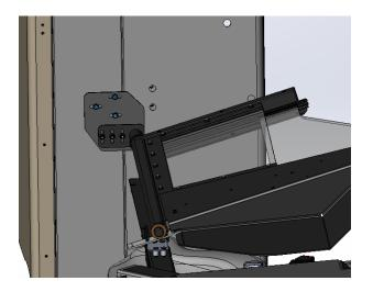
23. Using a level, make sure the hinge post is level front to back and side to side, adjust as needed by loosening the nuts and/or bolts and sliding in the needed direction.
